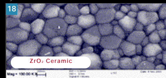
18 ZrO 2 Ceramic Zirconia structure, absence of glass phase and density, even though the photo is magnified ten times more than fig. 17
